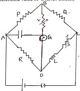
Circuit Diagram to determine value of r (A.C. Circuit)
