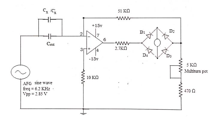
IC - 741- Operational Amplifier,  $C_{std}$  - Known capacitance,  $C_x$  - unknown Cylindrical capacitor, R- Known Resistances.
