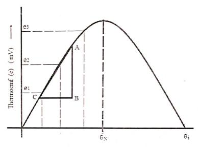
Note: With the existing laboratory facility it is difficult to reach neutral temperature  $\theta_N$ , ( $\theta_N$  for Cu-Fe Thermocouple is 270°C) and inversion temperature is  $2\theta_N$ . Therefore only initial part of the nature of graph is observed
