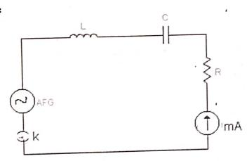
AFG: Audio Frequency Generator L: Inductance box C: Capacitance box R: Resistance box mA: Digital multimeter K: Plug key
