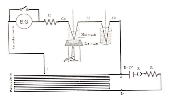
E = Regulated power supply; K= plug key;  $R_1$ = 2 K $\Omega$ ;  $R_2$ = 100 K $\Omega$ ; A to B= 10m wire of potentiometer; J= jockey; B.G= Ballistic Galvanometer
